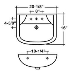
Dimensions of fixture are nominal and may vary within the range of tolerances established by ASME Standard A112.19.2. Dimensions and specifications subject to change without notice.
